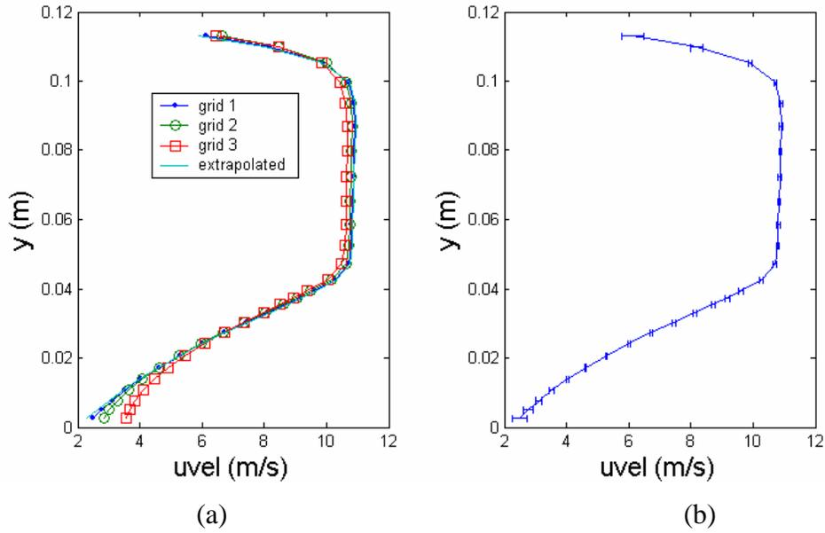
**Figure 1(a): Axial velocity profiles for a two-dimensional turbulent backward-facing-step flow calculation, Ref: Celik & Karatekin [1];**
