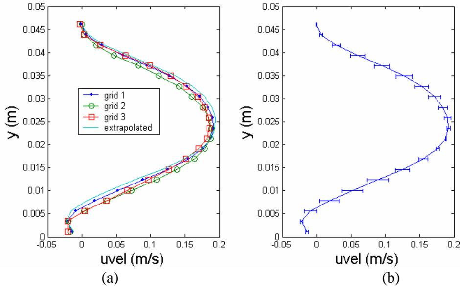
**Figure 2(a): Axial velocity profiles for a two-dimensional laminar backward-facing-step flow calculation, Ref: Celik & Badeau [1];**
